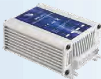
SR.202 Input V 20-35 Vdc - Output 13.6 Vdc Output: Amp. 20A - Eff. 90% Dim. 126x88x49 - vpe 1
