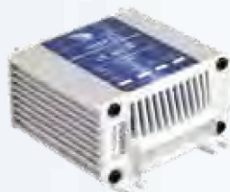
SR.212 Input V 9.0-18.0 Vdc - Output 24 Vdc Output: 170W - Amp. 7A - Eff. 90% Dim. 98x88x49 - vpe 1
