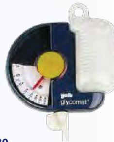
AP.180 Measuring range (20°C): 0 to -40°C WXhxD: 142 X 178 X 38 mm PLASTIC 1
