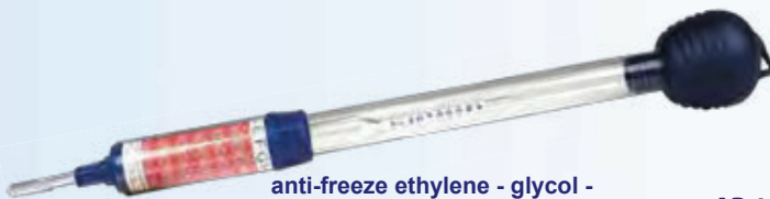
AP.181 - Measuring range (20°C): 0 to -50°C Temperature display: 2 to 74°C L: 360 mm - GLAS 1
