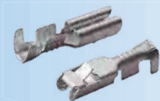
KV.118 female - 2.8 x 0.8 mm 0.5 - 1.0 mm 2
