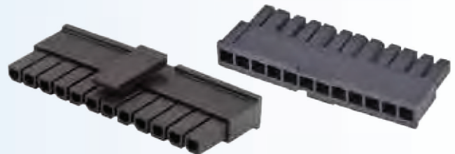
43645-1200 Micro-Fit 3.0 Receptacle Housing Single Row, 12 Circuits, UL 94V-0 vpe 10
