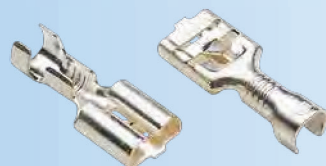
KV.120 (60838-1) female - 6.3 x 0.8 mm 0.5 - 1.0 mm 2
